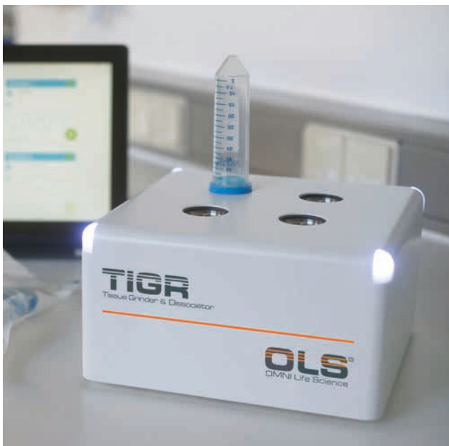
TIGR Tissue Grinder & Dissociator offers a fast and simple workflow from tissue to single cells
